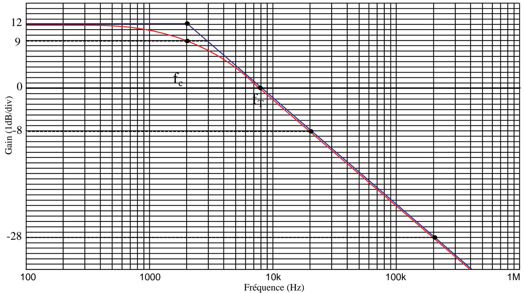
Exemple choisi :  $A = 4 \Leftrightarrow G(\text{BP}) = 12 \text{ dB}$  ;  $f_c = 2 \text{ kHz}$  ;  $f_T = 8 \text{ kHz}$
