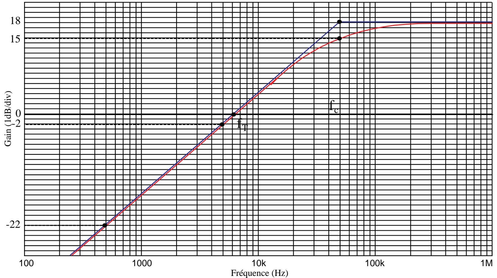
Exemple choisi :  $A = 8 \Leftrightarrow G(\text{BP}) = 18 \text{ dB}$  ;  $f_c = 50 \text{ kHz}$  ;  $f_T = 6 \text{ kHz}$
