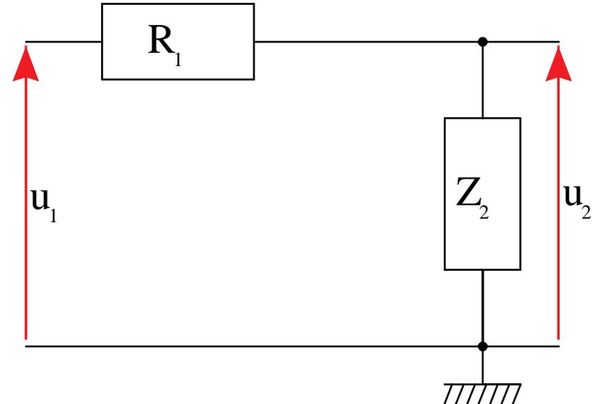
$$\underline{T}(j\omega) = \frac{R_2}{R_1 + R_2} \frac{1}{1 + j\omega C \frac{R_1 R_2}{R_1 + R_2}}$$
